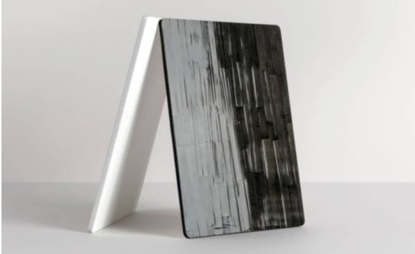
Fairmat's proprietary mechanical and robotic recycling technologies transform carbon fibre waste into CFRP chips, a second-generation carbon fibre that can be used in various applications. ©Alexandra de Cossette.
