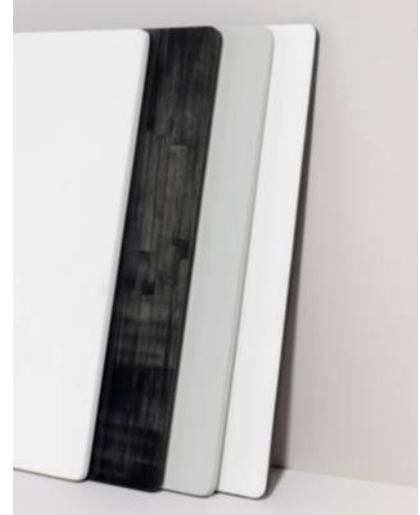
Fairmat's proprietary mechanical and robotic recycling technologies transform carbon fibre waste into CFRP chips, a second-generation carbon fibre that can be used in various applications. ©Alexandra de Cossette.
