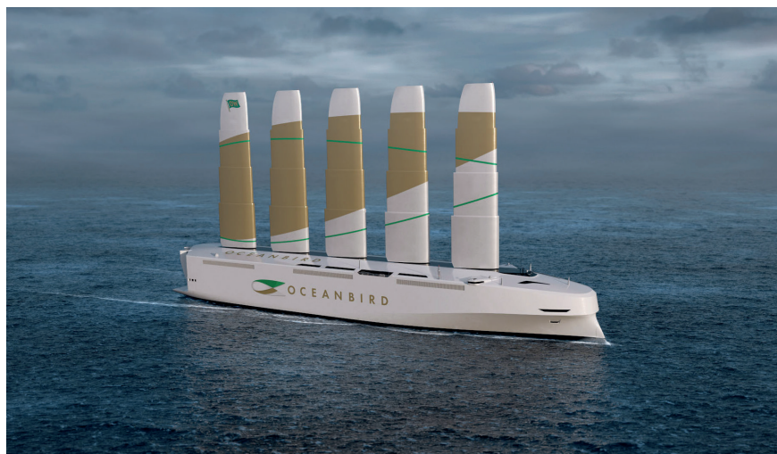
Announced last year, the Oceanbird vessel under development by Wallenius Marine to build a 200m wind-powered ro-ro, with wingsails made from composites and steel
