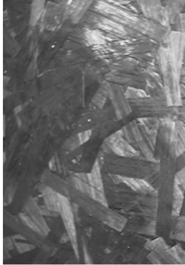
Figure 1: Sample of HexMC random chipped fiber distribution
