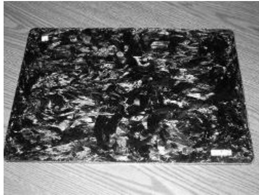
Figure 2: Producing a high-flow test panel
