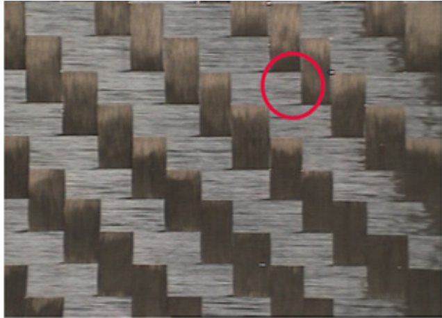
PrimeTex® 193 gsm, Twill 2/2, HS12K Open factor: 0.3%
