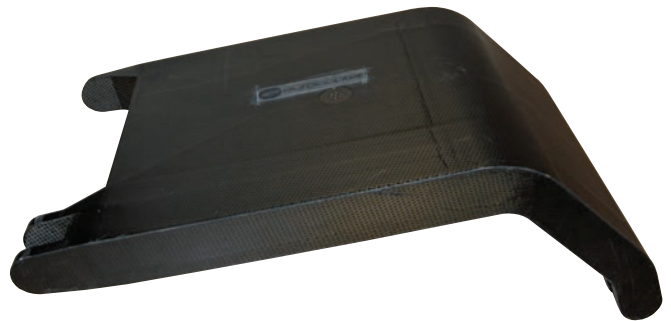
Figure 4: Airbus A380 door hinge arm manufactured by Airbus Helicopters using HexFlow® RTM6 resin and HexForce® G0926 carbon fibre fabric. There are 16 door hinge arms on each A380. As well as saving weight, they provide better thermal insulation in the cabin, reducing heat loss
