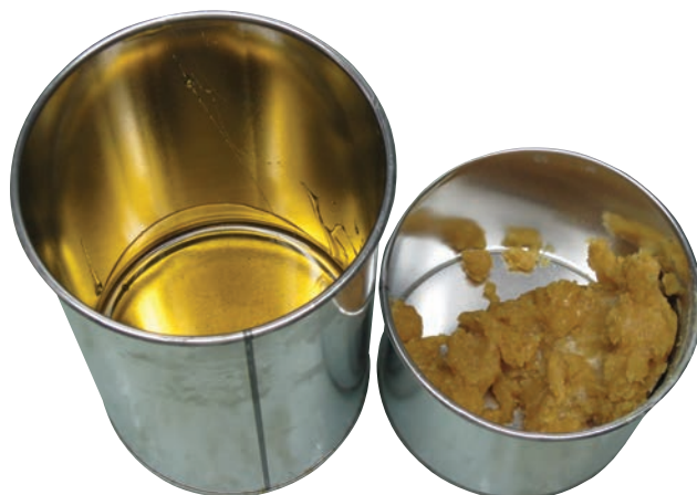
Figure 21: HexFlow® RTM6-2 Part A and Part B
