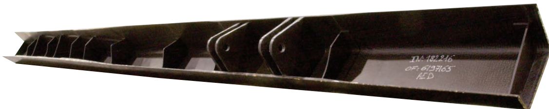
Figure 5: Airbus A380 aileron spar, manufactured by Airbus France (Nantes), using HexFlow®RTM6 resin and Injectex® woven carbon reinforcement
