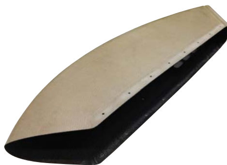
Figure 6: Embraer's Legacy 500 BizJet Horizontal Tail Plane Tip Fairing HexFlow®RTM6-2 resin and HexForce® G0926 carbon fibre fabric
