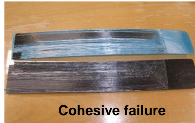
Good adhesion of infused glass on prepreg carbon laminate
