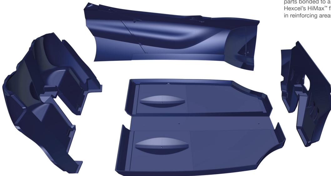
The chassis comprises five carbon composite parts bonded to a central aluminium spine. Hexcel's HiMax™ fabrics play an integral role in reinforcing areas of the floor.
