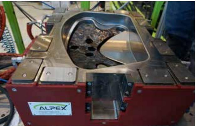
To meet these challenges, the partners selected Hexcel's version of carbon fibre SMC, HexMC®-i 2000 - the best-performing moulding compound currently on the market. It has been designed specifically to bridge the price–performance gap between conventional SMC and preangs, and is stiffer than steel at approximately a fifth of the density. Its mechanical performance is highly consistent.
