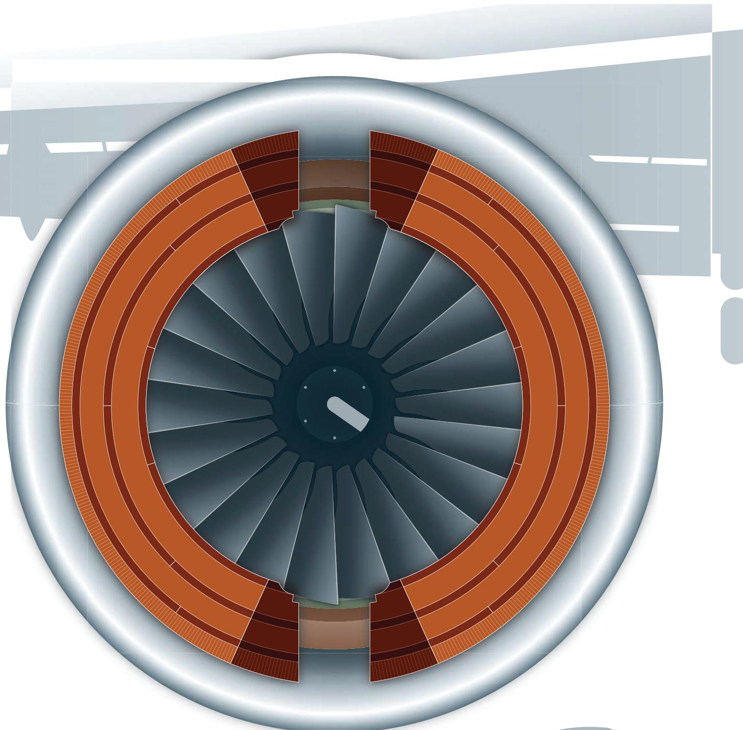
The cowling and fan duct sections surrounding a modern high-bypass airplane turbine engine are collectively referred to as the nacelle. The center image shows a nacelle cowl assembly. Honeycomb is used throughout the nacelle's construction, providing support that withstands vibration, high temperatures and offers sound attenuation.
