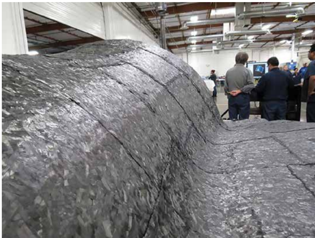
Figure 5: Plies of HexTool® applied to master using the tile concept.
