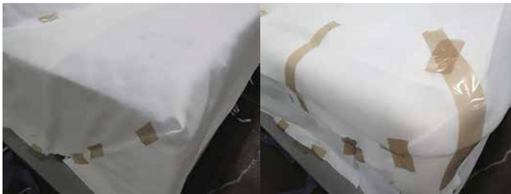
Figure 26: Ultraweave 1332 breather placed on top of solid FEP film with extra strips installed on corners and edges to protect final bag.
