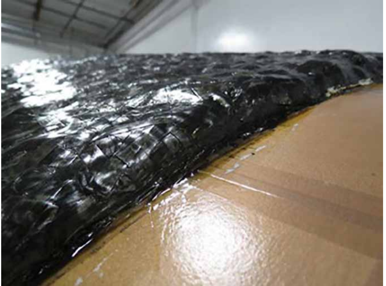
Figure 16: Seven debulked plies of HexTool® on an epoxy foam master with Tooltec release.
