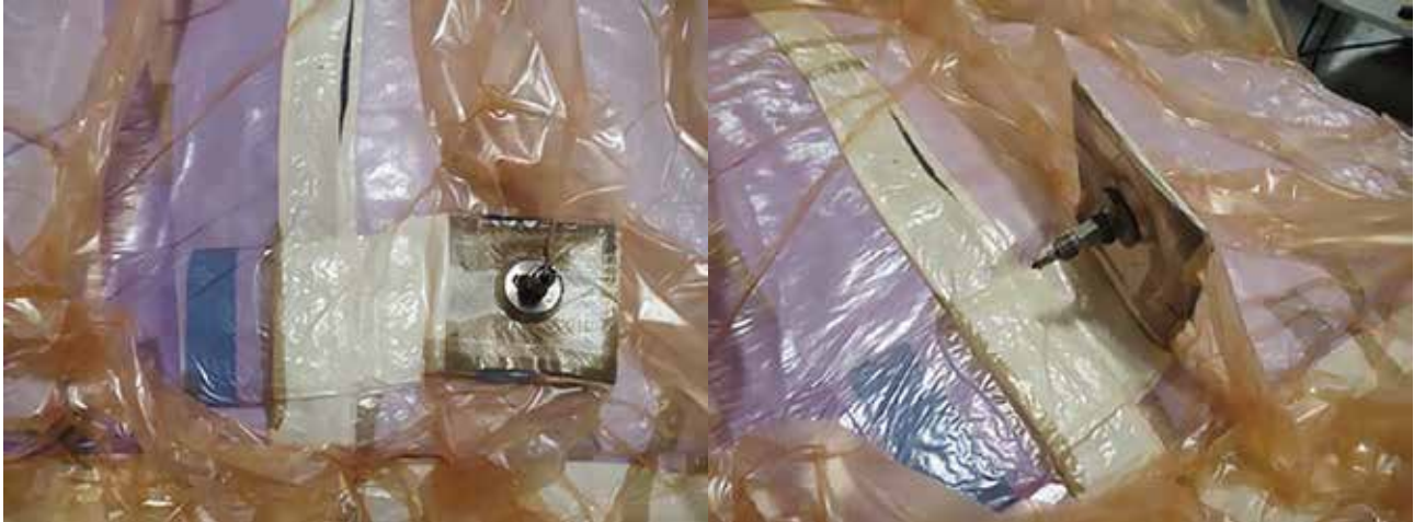
Figure 28: Vacuum port in bag pleat of final bag.
