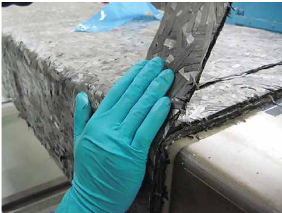
Figure 7: Application of warm HexTool® ply on an outside radius. Apply the material to one side and wrap carefully around the corner.
