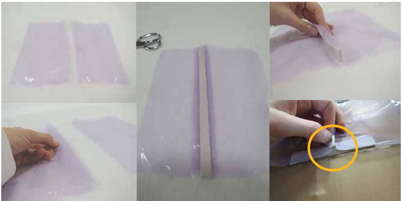
Figure 24: Example of preferred bag film seaming method.
