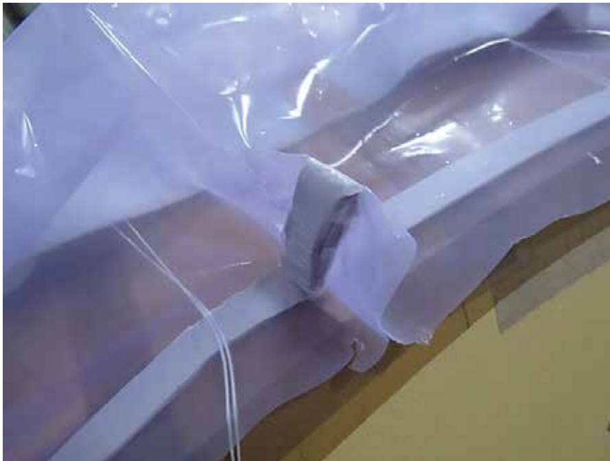
Figure 22: Solid FEP film inner bag installed on HexTool® tool and sealed. Note how breather string hangs outside of bag.
