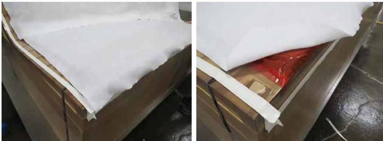
Figure 19: Application of first layer of breather over perforated FEP
