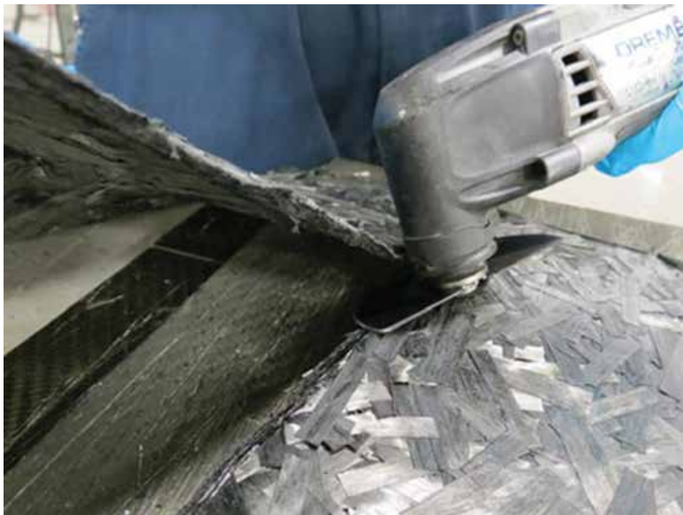
Figure 3: Chamfered ends of HexTool® plies cut at 30-45° with a vibratory saw. Pre-cut plies off of the master to avoid damage to the master.
