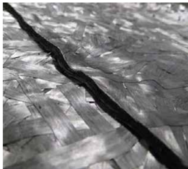
Figure 9: Circled area is at risk for filling with resin due to bridging of the next ply (left). The tile edge that was cut at 90° instead of 30-45° should be shaved or trimmed at an angle (right).
