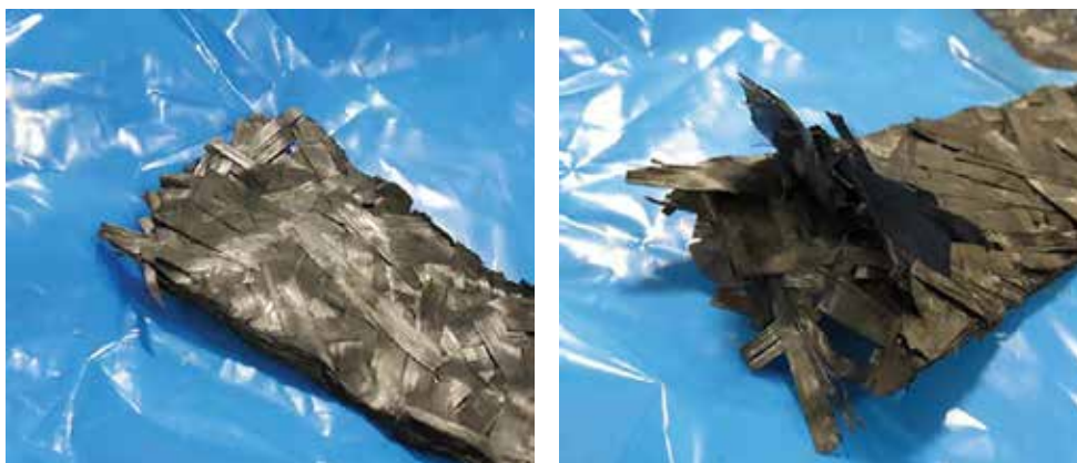
Figure 11: A HexTool® piece is peeled apart to use for patching.
