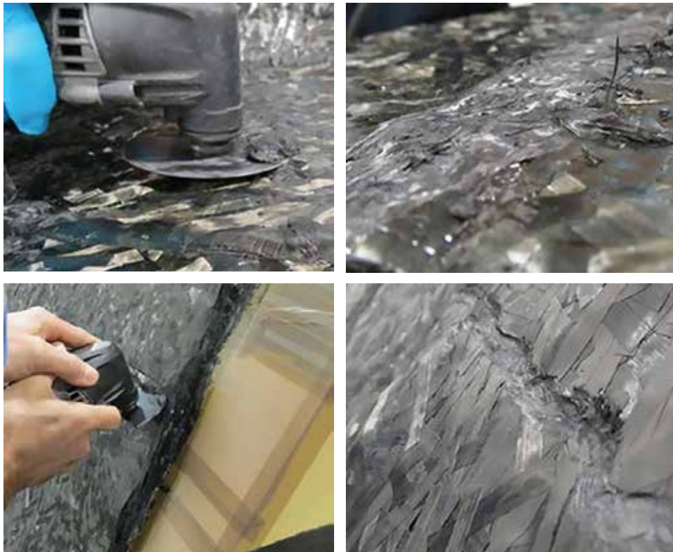
Figure 10: Examples of shaving and trimming material after it has been placed on a tool master (left) and finished appearance (right).
