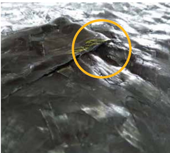
Figure 9: Circled area is at risk for filling with resin due to bridging of the next ply (left). The tile edge that was cut at 90° instead of 30-45° should be shaved or trimmed at an angle (right).
