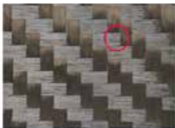
PrimeTex® 193 gsm, Twill 2/2, HS12K Open factor: 0.3%
