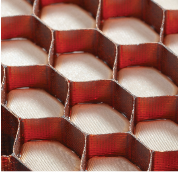
Non-Metallic HexWeb® Acousti-Cap® consists of permeable cap material embedded into a honeycomb core to create an acoustic septum.
