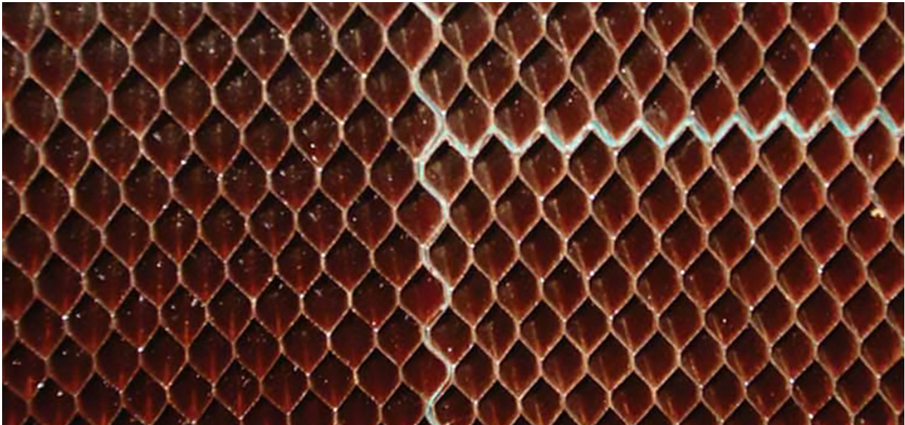
Seaming Technology Hexcel innovative seaming technology delivers a “spliceless” part for greater structural integrity.
