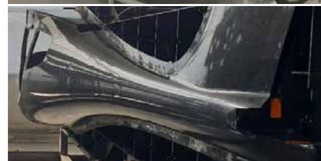
As more and more of its composite aircraft parts are transferred to prepreg technology, Flight Design is seeing the benefits of its switch to HexPly M79. Lay-up is cleaner and more precise, low temperature oven curing is quick and energy efficient, and the manufacturing process consistently outputs exceptionally high-quality laminates and components. The long-term strategy is to integrate HexPly M79 across the range, with Hexcel materials lightening the ultralight at Flight Design even further.
